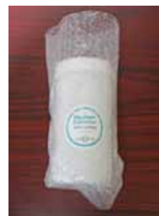
4. Carefully roll up sleeve, insert into canister and wrap OUTSIDE canister in bubble wrap
