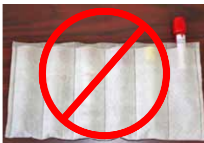
3b. NEVER INSERT DISCHARGE TUBE INTO TUBE SLEEVE. If used, the discharge tube should be discarded.
