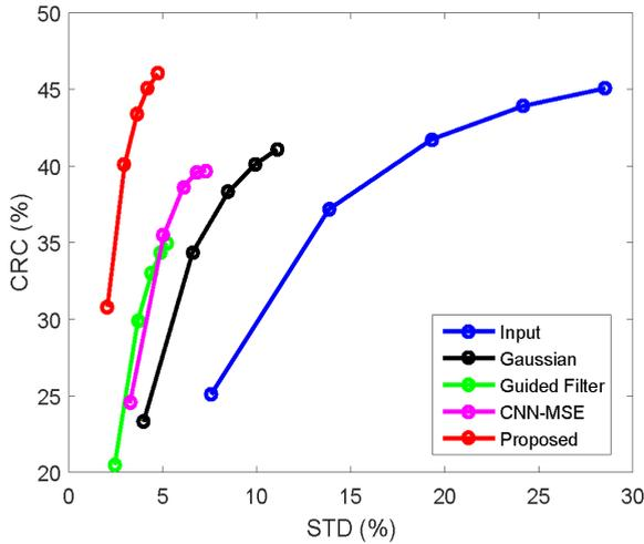
**FIGURE 11.** Plot of the CRC versus STD trade-off curves of slice 34 (generated with increasing MLEM iterations of 24, 48, 72, 96, and 120) obtained using: (i) Input, (ii) Gaussian, (iii) Guided Filter, (iv) CNN-MSE, and (v) Proposed.
