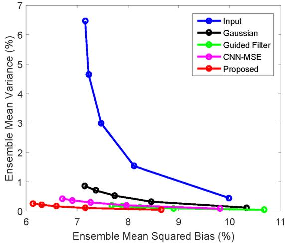
**FIGURE 12.** Plot of the ensemble variance versus ensemble means squared bias trade-off curves of slice 34 (generated with increasing MLEM iterations of 24, 48, 72, 96, and 120) obtained by using: (i) Input, (ii) Gaussian, (iii) Guided Filter, (iv) CNN-MSE, and (v) Proposed.
