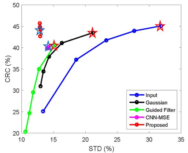
**FIGURE 13.** The CRC between the gray matter and the white matter versus the STD in white matter curves of slice 34 by varying the main parameters of each method, for (i) Input (increasing iterations), (ii) Gaussian (increasing FWHM), (iii) Guided Filter (increasing windows size), (iv) CNN-MSE (increasing trained iterations), and (v) Proposed (increasing trained iterations). The point with similar CRC value labeled by star markers will be used for visual evaluation in Fig. 15.
