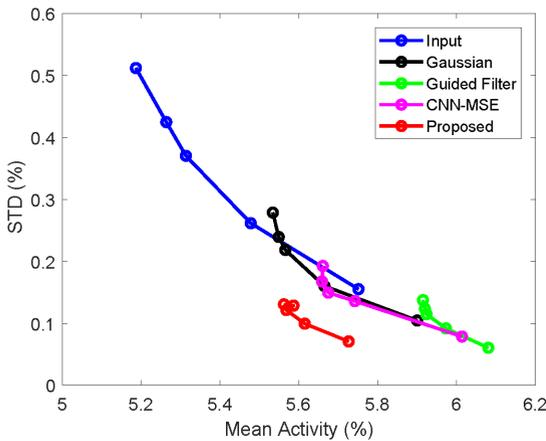
**FIGURE 18.** Plot of the STD versus Mean Activity trade-off curves of slice 16 of clinical brain test data changing with the iteration number. Thirty square ROIs with the size of  $12 \times 12 \text{ mm}^2$  were selected, as generated by adding ten ROIs randomly based on the twenty ROIs from Fig. 17.
