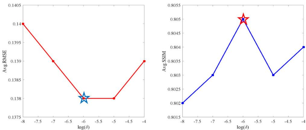
**FIGURE 8.** Plots of the average RMSEs (left) and average SSIMs (right) on the simulation test data by changing the parameter  $\delta$  with  $10^{-4}$ ,  $10^{-5}$ ,  $10^{-6}$ ,  $10^{-7}$ ,  $10^{-8}$  when the  $w_1$  was set to be 0.0005, the  $w_2$  was 0.075. The parameter  $\delta$  chosen in the manuscript was marked by ☆.
