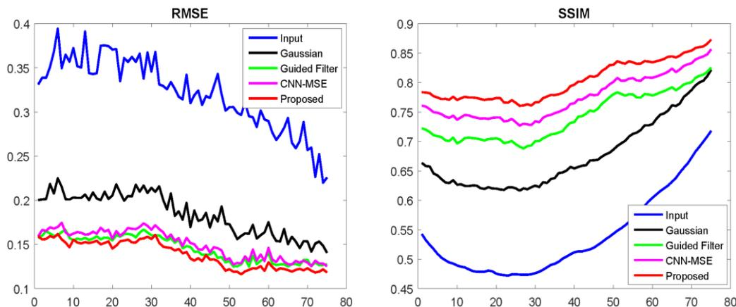
FIGURE 9. The RMSE and SSIM of each test resulting image (a total of 75 images) using different denoising algorithms (Gaussian filter, guided filter, CNN-MSE, and the proposed method).
