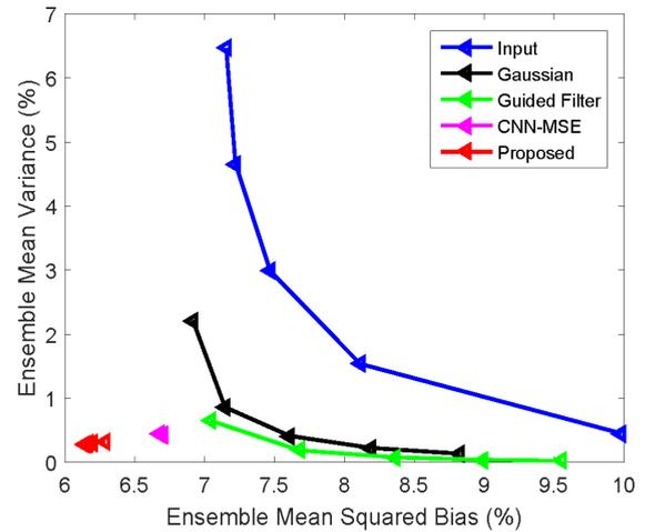
**FIGURE 14.** Plot of the ensemble variance versus ensemble means squared bias trade-off curves of slice 34 by varying the main parameters of each method, for (i) Input (increasing iterations), (ii) Gaussian (increasing FWHM), (iii) Guided Filter (increasing windows size), (iv) CNN-MSE (increasing trained iterations), and (v) Proposed (increasing trained iterations).
