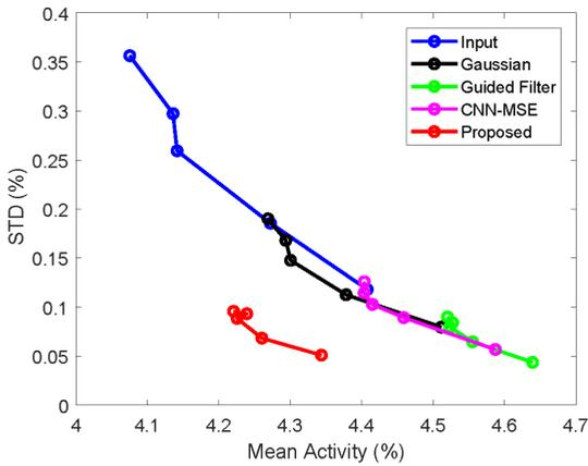
**FIGURE 17.** Plot of the STD versus Mean Activity trade-off curves of slice 16 of clinical brain test data changing with the iteration number (increasing iteration of 24, 48, 72, 96, and 120) obtained using: (i) Input, (ii) Gaussian, (iii) Guided Filter, (iv) CNN-MSE, and (v) Proposed. Twenty ROIs with the size of  $12 \times 12 \text{ mm}^2$  were randomly selected.
