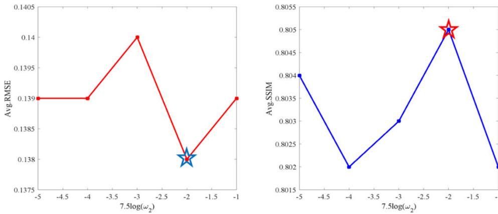
**FIGURE 7.** Plots of the average RMSEs (left) and average SSIMs (right) on the simulation test data by changing the parameter  $w_2$  with 0.75, 0.075, 0.0075, 0.00075, 0.000075 when the  $w_1$  was 0.0005, the  $\delta$  was  $10^{-6}$ . The parameter  $w_2$  chosen in the manuscript was marked by ☆.
