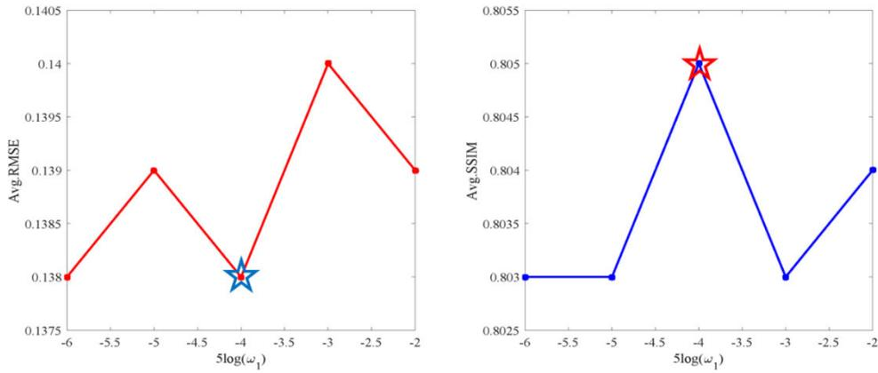
**FIGURE 6.** Plots of the average RMSEs (left) and average SSIMs (right) on the simulation test data by changing the parameter  $w_1$  with 0.05, 0.005, 0.0005, 0.00005, and 0.000005 when the  $w_2$  was 0.075, the  $\delta$  was  $10^{-6}$ . The parameter  $w_1$  chosen in the manuscript was marked by ☆.
