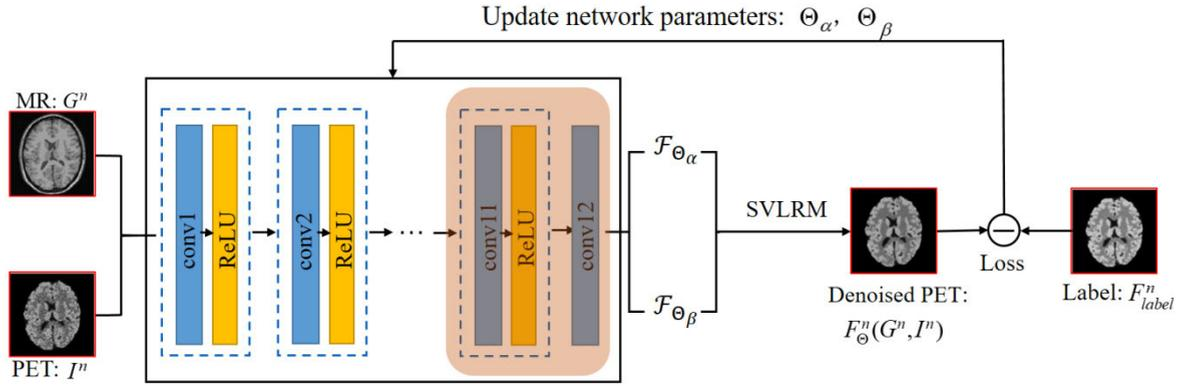
FIGURE 1. Schematic of the proposed deep learning-based joint filtering framework.
