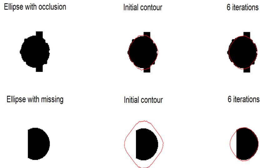
**Figure 6.** Experiments on ellipse synthetic image. Left column is original image, middle column is initial contour, right column is segmentation results. The first row is experiment on ellipse with occlusion, the second row is experiment on ellipse with missing.
