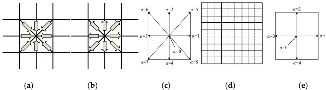
**Figure 3.** Explanation of the lattice Boltzmann (LB) method for image processing. (a) Collision process; (b) streaming process; (c) D2Q9 structure; (d) sub-pixel denoted by dotted box and pixel denoted by solid box; (e) D2Q5 structure.
