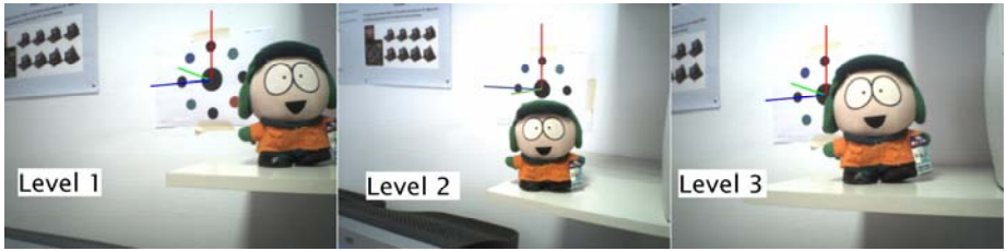
Fig. 4. Examples of several occlusion levels. As we can see, the landmark reference system retroprojected on the image according to the calculated camera positioning.
