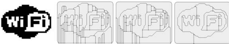
Fig. 2. A digital image I , and boundary graphs \bar{G}_6 , \bar{G}_{10} and \bar{G}_{16} of the pyramid of I
