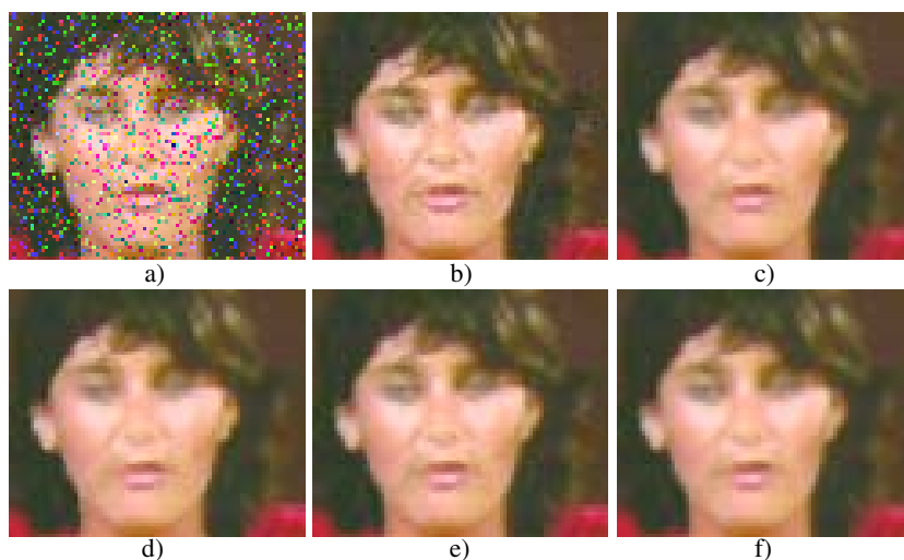
Fig. 3. Subjective visual qualities of restored 10th frame of “Miss America” video sequence, a) Zoomed image region contaminated by impulsive noise of 15% intensity , b) Designed 3D-FD, c) 3D-VMF, d) 3D-GVDF, e) 3D-AVDATM, f) 3D-ATM
