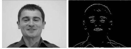
Fig. 3.1. a) Gray scale image, b) Edge detection with a Sobel filter and a T = 0.5804 thresholding
