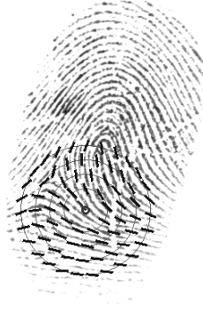
Fig. 1. A representation of the minutia descriptor proposed in [11]
