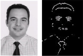
Fig. 4.2. Edge detection with thresholding T = 0.5608
