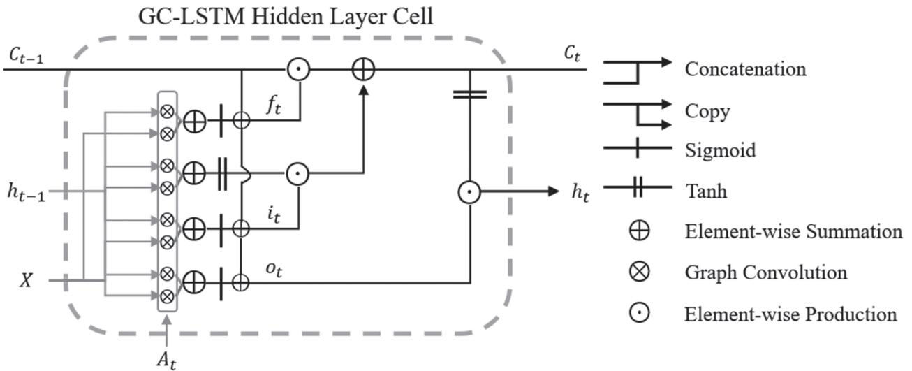
Figure 2. GC-LSTM hidden cell in detail. Each cell has two sources of input, the present ( $A_t$  and  $X$ ) and the recent past ( $h_{t-1}$  and  $C_{t-1}$ ). Output sequence ( $h_t | t = 1, 2, \dots, T$ ) was then treated as feature maps for following layers.
