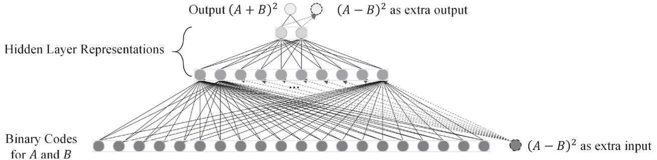
Figure 8. Network design for synthetic experiment to illustrate the effectiveness of assistant task learning. The classification model is composed of three fully connected layers. Number of node here represents the dimension of features.
